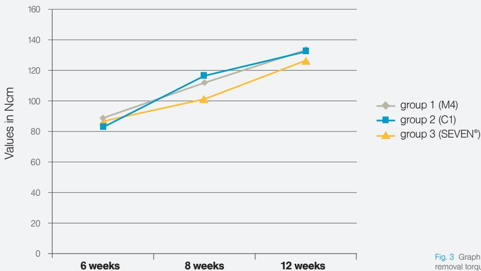
Fig. 3 Graph showing the evolution of the removal torque values.
